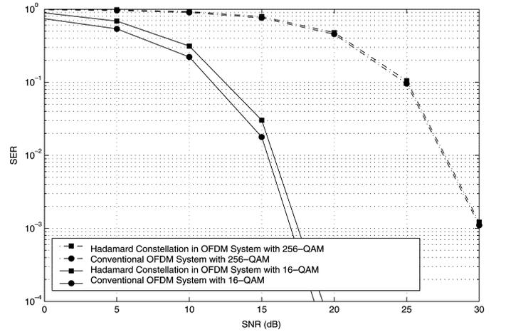
Fig. 7. SER comparison for the proposed method in a 256-channel OFDM system employing 256-QAM and 16-QAM constellation.
