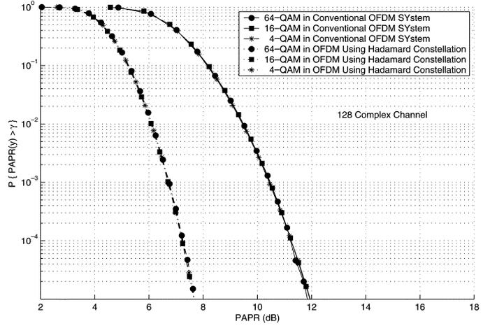
Fig. 6. CCDF of PAPR for a Hadamard constellation in a 128-channel OFDM system employing different QAM constellations and  $L = 1$ .
