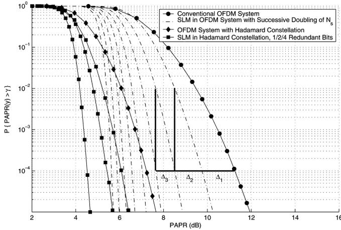
Fig. 9. CCDF of PAPR in a 128-channel OFDM system with SLM method using different number of redundant bits  $L = 1$ .
