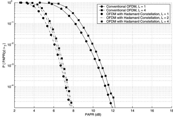
Fig. 4. CCDF of PAPR for a Hadamard constellation with different oversampling factors (128-channel OFDM system with 16-QAM constellation).
