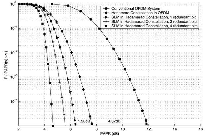
Fig. 8. CCDF of PAPR by SLM method based on Hadamard constellation in a 128-channel OFDM system employing 16-QAM constellation.
