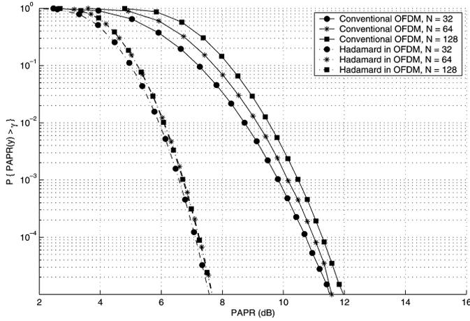
Fig. 5. CCDF of PAPR for a Hadamard constellation in an  $N$ -channel OFDM system employing 16-QAM constellation and  $L = 1$ .
