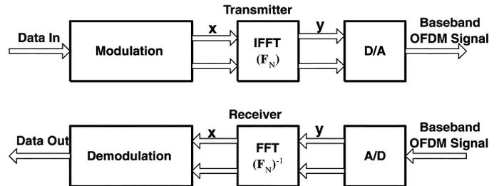
Fig. 1. Basic OFDM transmitter and receiver.
