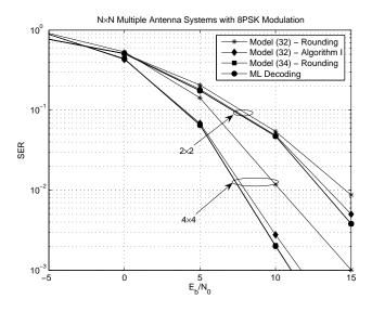
Fig. 3. Performance of the proposed model (32) and (34) in a MIMO system with N transmit and N receive antennas employing 8-PSK
