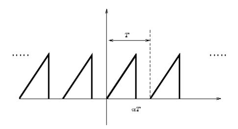
5.1. Find the autocorrelation function the power spectral density and the total power of this signal
