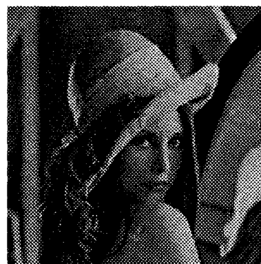
Figure 7: Turbo Decoder Output Using the Priority based Mapping Method (110 bpb, PSNR=30.85 dB)
