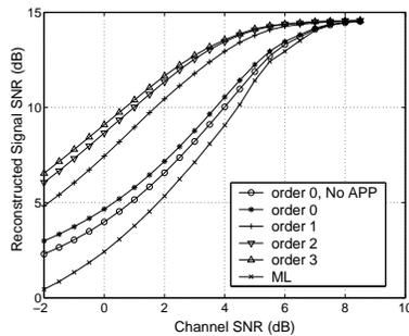
**Fig. 2.** Performance of the instantaneous MMSE decoder when different levels of residual redundancy is exploited at the decoder
